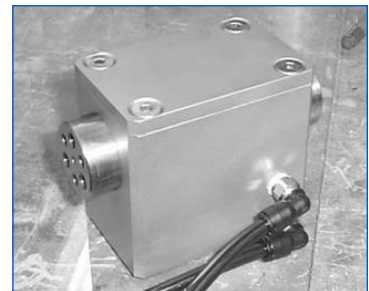
Internally sealed, stainless steel submersible gripper
